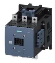
power contactor, AC-3e/AC-3 400 A, 200 kW / 400 V AC (50-60 Hz) / DC Uc: 96-127 V PLC input 24 V DC 3-pole, auxiliary contacts 2 NO + 2 NC drive: electronic main circuit: busbar control and auxiliary circuit: spring-loaded terminal
