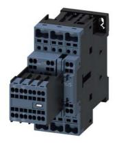
power contactor, AC-3e/AC-3, 38 A, 18.5 kW / 400 V, 3-pole, 24 V AC, 50 Hz, auxiliary contacts: 2 NO + 2 NC, spring-loaded terminal, size: S0, removable auxiliary switch
