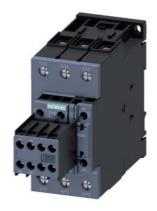
power contactor, AC-3e/AC-3, 80 A, 37 kW / 400 V, 3-pole, 42 V AC, 50 Hz, auxiliary contacts: 2 NO + 2 NC, screw terminal, size: S2, removable auxiliary switch
