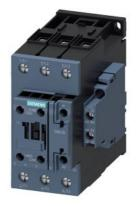
power contactor, AC-3e/AC-3, 65 A, 30 kW / 400 V, 3-pole, 20-33 V AC/DC, 50/60 Hz, with integrated varistor, auxiliary contacts: 2 NO + 2 NC, screw terminal, size: S2, lateral auxiliary switch
