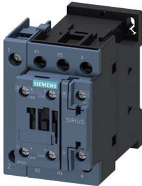
power contactor, AC-3, 25 A, 11 kW / 400 V, 4-pole, 24 V AC, 50/60 Hz, main contacts: 2 NO + 2 NC, auxiliary contacts: 1 NO + 1 NC, screw terminal, size: S0
