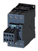
power contactor, AC-3e/AC-3, 65 A, 30 kW / 400 V, 3-pole, 83-155 V AC/DC, 50/60 Hz, with integrated varistor, auxiliary contacts: 2 NO + 2 NC, screw terminal, size: S2, removable auxiliary switch
