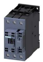
power contactor, AC-3e/AC-3, 51 A, 22 kW / 400 V, 3-pole, 110 V AC, 50 Hz / 120 V, 60 Hz, auxiliary contacts: 1 NO + 1 NC, main circuit: screw terminal, control and auxiliary circuit: spring-loaded terminal, size: S2
