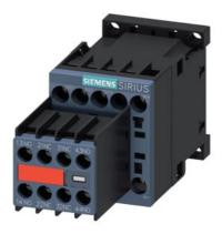
power contactor, AC-3e/AC-3, 12 A, 5.5 kW / 400 V, 3-pole, 24 V DC, auxiliary contacts: 2 NO + 2 NC, screw terminal, size: S00, captive auxiliary switch
