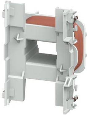
magnetic coil 200 V AC, 50/60 Hz / 220 V, 60 Hz, for contactors 3RT2325-.A, 3RT2.26-.A, 3RT2.27-.A and 3RT2028-.A
