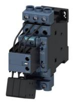
capacitor contactor, AC-6b 33 kVAr, / 400 V, 3-pole, 24 V DC, auxiliary contacts: 1 NO + 2 NC, screw terminal, size: S0  $\,$
