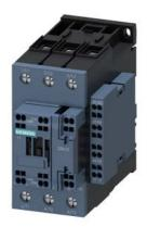
power contactor, AC-3e/AC-3, 51 A, 22 kW / 400 V, 3-pole, 230 V AC, 60 Hz, auxiliary contacts: 2 NO + 2 NC, main circuit: screw terminal, control and auxiliary circuit: spring-loaded terminal, size: S2, lateral auxiliary switch
