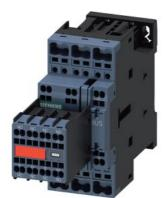
power contactor, AC-3e/AC-3, 32 A, 15 kW / 400 V, 3-pole, 110 V AC, 50 Hz / 120 V, 60 Hz, auxiliary contacts: 2 NO + 2 NC, spring-loaded terminal, size: S0, captive auxiliary switch, no surge suppressor retrofittable
