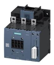
power contactor, AC-3e/AC-3 185 A, 90 kW / 400 V AC (50-60 Hz) / DC Uc: 96-127 V PLC input 24 V DC 3-pole, auxiliary contacts 1 NO + 1 NC drive: electronic main circuit: busbar control and auxiliary circuit: screw terminal with remaining lifetime indicator
