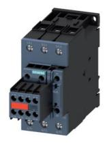
power contactor, AC-3e/AC-3, 41 A, 18.5 kW / 400 V, 3-pole, 20-33 V AC/DC, 50/60 Hz, with integrated varistor, auxiliary contacts: 2 NO + 2 NC, screw terminal, size: S2, captive auxiliary switch
