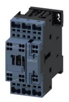
power contactor, AC-3e/AC-3, 32 A, 15 kW / 400 V, 3-pole, 208 V AC, 50/60 Hz, auxiliary contacts: 1 NO + 1 NC, spring-loaded terminal, size: S0
