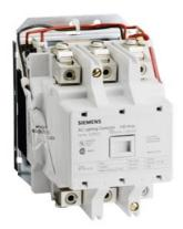
Mechanically held lighting contactor, Contactor amp rating 100A, 0 N.C. / 3 N.O. poles, 24VAC 60HZ coil, Non-combination type, Enclosure NEMA type (open), No enclosure
