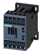
power contactor, AC-3e/AC-3, 9 A, 4 kW / 400 V, 3-pole, 24 V DC, with integrated diode, auxiliary contacts: 1 NO, spring-loaded terminal, size: S00
