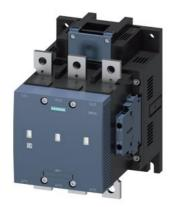
vacuum contactor AC-3e/AC-3 225 A, 110 kW / 400 V, 3-pole, Uc: 575-600 V AC(50-60 Hz) / DC drive: conventional auxiliary contacts 2 NO + 2 NC main circuit: busbar control and auxiliary circuit: screw terminal
