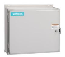
Mechanically held lighting contactor, Contactor amp rating 30A, 0 N.C. / 6 N.O. poles, 220VAC 50HZ/240VAC 60HZ coil, Non-combination type, Enclosure NEMA type 12, Dust/drip proof for indoors
