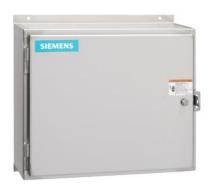
Mechanically held lighting contactor, Contactor amp rating 60A, 0 N.C. / 8 N.O. poles, 110VAC 50HZ/120VAC 60HZ coil, Non-combination type, Enclosure NEMA type 12, Dust/drip proof for indoors
