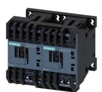
reversing contactor assembly, AC-3e/AC-3, 12 A, 5.5 kW / 400 V, 3-pole, 48 V AC, 50/60 Hz, spring-loaded terminal, electrical and mechanical interlock
