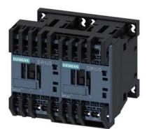
reversing contactor assembly, AC-3e/AC-3, 12 A, 5.5 kW / 400 V, 3-pole, 110 V AC, 50/60 Hz, spring-loaded terminal, electrical and mechanical interlock
