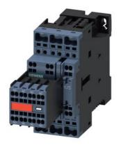
power contactor, AC-3e/AC-3, 17 A, 7.5 kW / 400 V, 3-pole, 24 V DC, with plugged-in varistor, auxiliary contacts: 2 NO + 2 NC, spring-loaded terminal, size: S0, captive auxiliary switch
