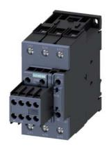
power contactor, AC-3e/AC-3, 80 A, 37 kW / 400 V, 3-pole, 110 V AC, 50 Hz, auxiliary contacts: 2 NO + 2 NC, screw terminal, size: S2, removable auxiliary switch
