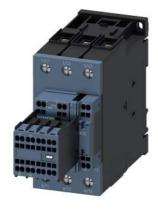
traction contactor, AC-3e/AC-3, 51 A, 22 kW / 400 V, 3-pole, 110 V DC, 0.7-1.25 $^{\star}$  Us, electronic drive, with integrated varistor, auxiliary contacts: 2 NO + 2 NC, main circuit: screw terminal, control and auxiliary circuit: spring-loaded terminal, size: S2, removable auxiliary switch
