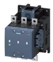
vacuum contactor AC-3e/AC-3 225 A, 110 kW / 400 V, 3-pole, Uc: 500-550 V AC(50-60 Hz) / DC drive: conventional auxiliary contacts 2 NO + 2 NC main circuit: busbar control and auxiliary circuit: screw terminal
