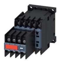
contactor relay, 4 NO + 4 NC, 480 V AC, 50 / 60 Hz, size S00, ring cable lug connection, captive auxiliary switch
