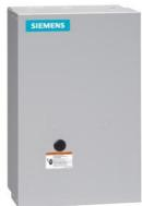
Mechanically held lighting contactor, Contactor amp rating 100A, 0 N.C. / 4 N.O. poles, 24VAC 60HZ coil, Non-combination type, Enclosure NEMA type 1, Indoor general purpose use
