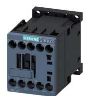
power contactor, AC-3e/AC-3, 16 A, 7.5 kW / 400 V, 3-pole, 60 V DC, auxiliary contacts: 1 NC, screw terminal, size: S00  $\,$
