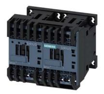
reversing contactor assembly, AC-3e/AC-3, 12 A, 5.5 kW / 400 V, 3-pole, 24 V DC, spring-loaded terminal, electrical and mechanical interlock, with voltage tap for  $3 \rm RA27$
