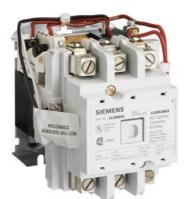
Mechanically held lighting contactor, Contactor amp rating 60A, 0 N.C. / 4 N.O. poles, 208VAC 60HZ coil, Non-combination type, Enclosure NEMA type (open), No enclosure
