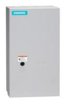
Mechanically held lighting contactor, Contactor amp rating 200A, 0 N.C. / 4 N.O. poles, 277VAC 60HZ coil, Non-combination type, Enclosure NEMA type 1, Indoor general purpose use
