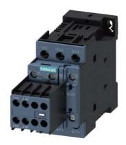
power contactor, AC-3e/AC-3, 25 A, 11 kW / 400 V, 3-pole, 48 V DC, auxiliary contacts: 2 NO + 2 NC, screw terminal, size: S0, removable auxiliary switch
