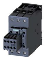
power contactor, AC-3e/AC-3, 65 A, 30 kW / 400 V, 3-pole, 400 V AC, 50 Hz / 400-440 V, 60 Hz, auxiliary contacts: 2 NO + 2 NC, screw terminal, size: S2, removable auxiliary switch
