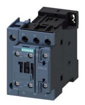
power contactor, AC-3, 25 A, 11 kW / 400 V, 4-pole, 12 V DC, main contacts: 2 NO + 2 NC, auxiliary contacts: 1 NO + 1 NC, screw terminal, size: S0
