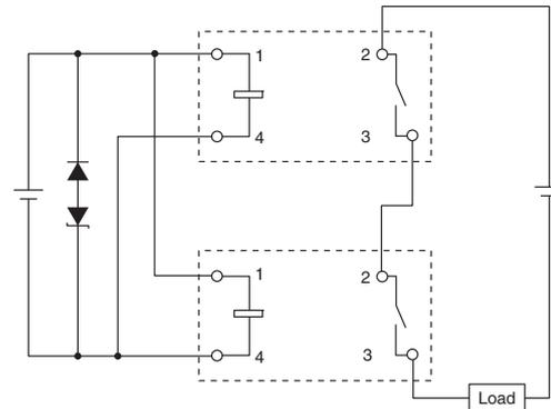
Note. The diode and zener diode are for the absorption of coil surge. (The coil does not have a polarity.)
