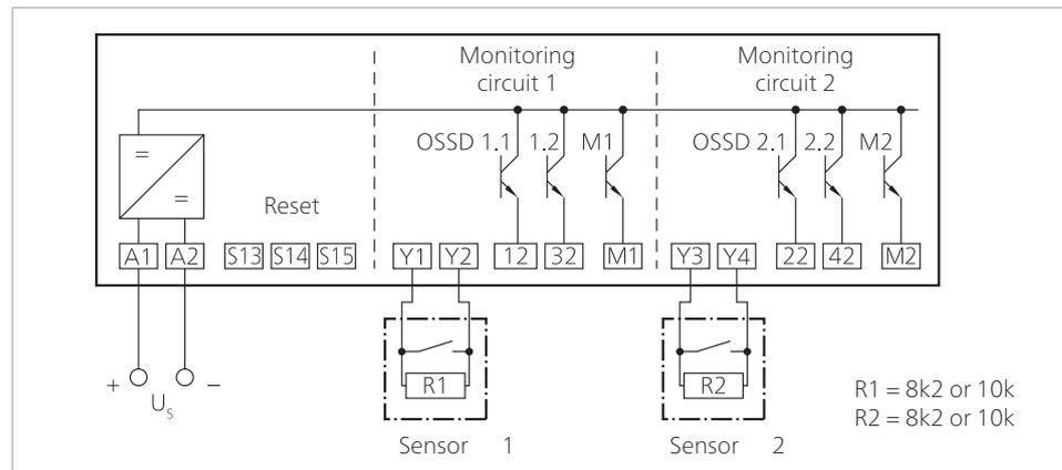
OSSDs 1.1, 1.2, 2.1 and 2.2 are semiconductor outputs (PNP) and short-circuit-proof. In the HIGH state (ON state), the voltage  $U_s - 0.7\text{ V}$  is applied, depending on the load and supply voltage.
