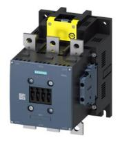
power contactor, AC-3e/AC-3 265 A, 132 kW / 400 V AC (50-60 Hz) / DC 200-277 V x (0.8-1.1) F-PLC input 24 V DC 3-pole, auxiliary contacts 2 NO + 2 NC drive: electronic main circuit: busbar control and auxiliary circuit: screw terminal
