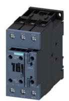
traction contactor, AC-3e/AC-3, 41 A, 18.5 kW / 400 V, 3-pole, 24 V DC, 0.7-1.25\* Us, electronic drive, with integrated varistor, auxiliary contacts: 1 NO + 1 NC, screw terminal, size: S2
