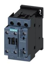
power contactor, AC-3e/AC-3, 25 A, 11 kW / 400 V, 3-pole, 24 V AC, 50 Hz, auxiliary contacts: 1 NO + 1 NC, screw terminal, size: S0, upright mounting position
