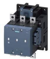
vacuum contactor AC-3e/AC-3 300 A, 160 kW / 400 V, 3-pole, Uc: 23-26 V AC(50-60 Hz) / DC drive: conventional auxiliary contacts 2 NO + 2 NC main circuit: busbar control and auxiliary circuit: screw terminal
