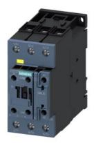
power contactor, AC-3e/AC-3, 80 A, 37 kW / 400 V, 3-pole, 21-33 V AC/DC, 50/60 Hz, with integrated varistor, auxiliary contacts: 1 NC, screw terminal, size: S2, F-PLC-IN
