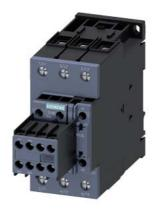
power contactor, AC-3e/AC-3, 41 A, 18.5 kW / 400 V, 3-pole, 24 V AC, 50/60 Hz, auxiliary contacts: 2 NO + 2 NC, screw terminal, size: S2, removable auxiliary switch
