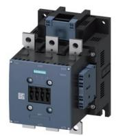
power contactor, AC-3e/AC-3 265 A, 132 kW / 400 V AC (50-60 Hz) / DC Uc: 23-26 V 3-pole, auxiliary contacts 2 NO + 2 NC drive: conventional main circuit: busbar control and auxiliary circuit: spring-loaded terminal
