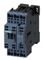
traction contactor, AC-3e/AC-3, 32 A, 15 kW / 400 V, 3-pole, 125 V DC, 0.7-1.25\* Us, electronic drive, with integrated varistor, auxiliary contacts: 1 NO + 1 NC, spring-loaded terminal, size: S0
