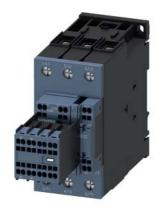
traction contactor, AC-3e/AC-3, 51 A, 22 kW / 400 V, 3-pole, 24 V DC, 0.7-1.25\* Us, electronic drive, with integrated varistor, auxiliary contacts: 2 NO + 2 NC, main circuit: screw terminal, control and auxiliary circuit: spring-loaded terminal, size: S2, removable auxiliary switch
