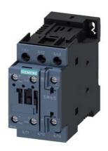
power contactor, AC-3e/AC-3, 25 A, 11 kW / 400 V, 3-pole, 24 V DC, auxiliary contacts: 1 NO + 1 NC, screw terminal, size: S0, communication-capable
