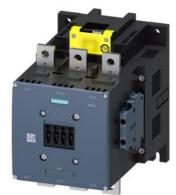
power contactor AC-1 690 A / 690 V / 40 °C 3-pole, Uc: 200-277 V AC(50-60 Hz) / DC F-PLC input 24 V DC drive: electronic auxiliary contacts 2 NO + 2 NC main circuit: busbar control and auxiliary circuit: screw terminal
