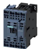
contactor AC-1, 50 A, 400 V / 40  $^\circ$ C, 4-pole, 24 V DC, auxiliary contacts: 1 NO + 1 NC, spring-loaded terminal, size: S0
