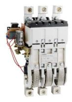
Mechanically held lighting contactor, Contactor amp rating 300A, 0 N.C. / 2 N.O. poles, 208VAC 60HZ coil, Non-combination type, Enclosure NEMA type (open), No enclosure
